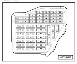
From fuse number 23 upwards the fuses in the fuse box are designated as 223 etc. in the Current Flow Diagram.
